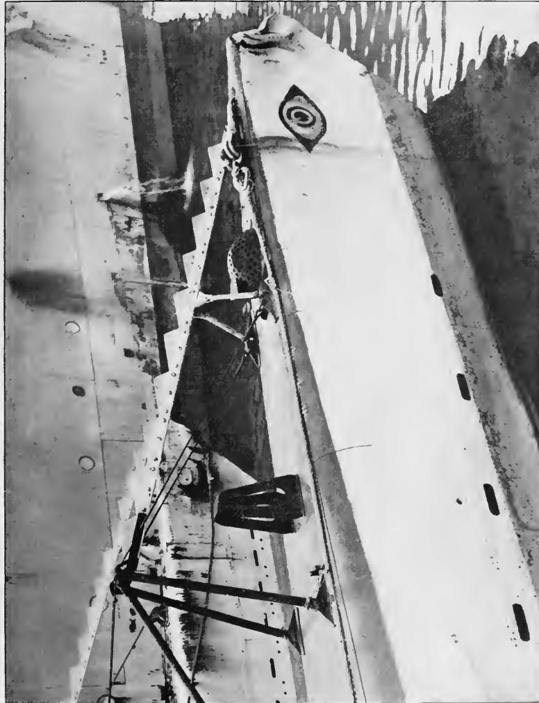
GERMAN U-BOAT SHOWING SAW-TEETH ON THE BOW USED FOR CUTTING NETS.
